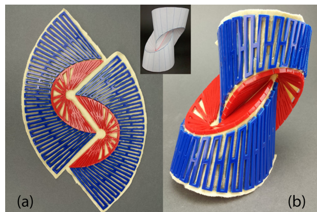
Fig. 16 Crashing volcanoes transitioned from paper (origami model is shown in the inset) to acrylic with a fabric backing in its (a) flat state and (b) deployed state
